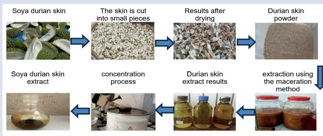
Figure 1. Process of collecting, processing and extracting Soya durian skin using 96% ethanol.
