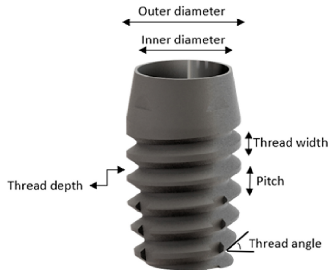
Figure 4: Geometrical features of the thread. CAD files realized in SolidWorks 2022.
