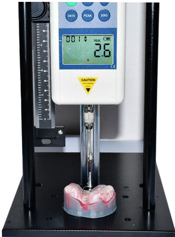
Figure 3: A moulding plate and cast with soft gum were placed on a traction device to investigate retention force.
