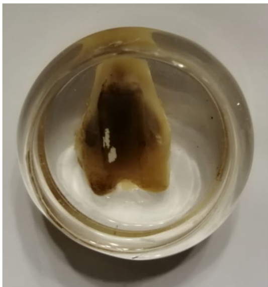
Figure 3: Rabbit femur head embedded in PMMA for preparation of undecalcified sections.
