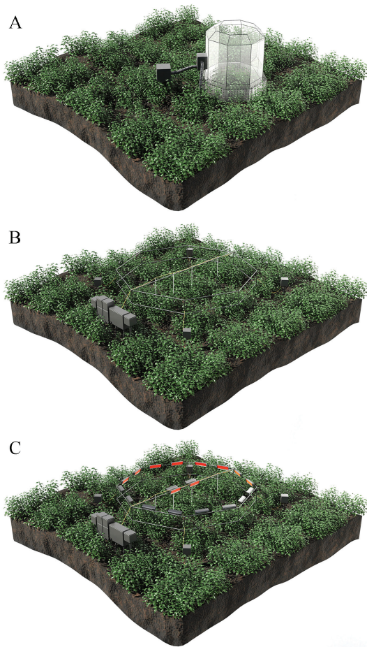
FIGURE 2 Platforms for assessing plant growth and yield in controlled environments: (A) open-top chamber (OTC), (B) free-air carbon dioxide enrichment (FACE), (C) temperature free-air carbon dioxide enrichment (T-FACE).
