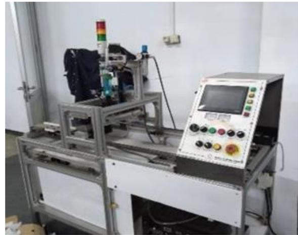
Gambar 1. Mesin plasma lucutan korona
