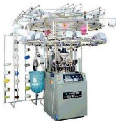
Gambar 8. Mesin rajut bundar *seamless single knit*
