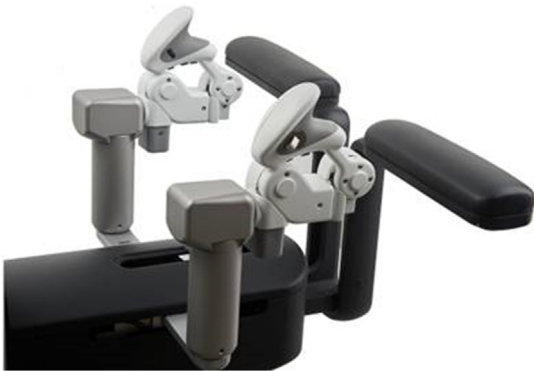
Fig. 4. Hominis Joysticks™ components: rigid section (shaft) and a flexible section; the latter is composed of three joints, according to the design of the human arm: Shoulder, Elbow, and Wrist.
