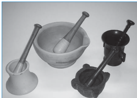
Figure 2.12 Mortars and pestles. (Left to right) ceramic pill mortar and pestle, composition mortar and pestle, stone mortar with a metal and wooden pestle, bell-metal mortar and pestle.
