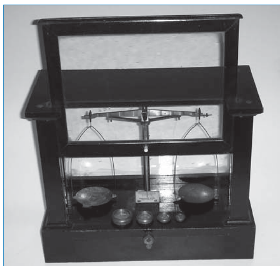
Figure 2.10 Chemical scales, made by Becker and Sons, Rotterdam, nineteenth century.
